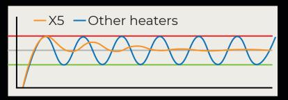
The graph above shows that X5 eliminates constantly oscillating temperatures by tuning combustion intensity to the situation.
